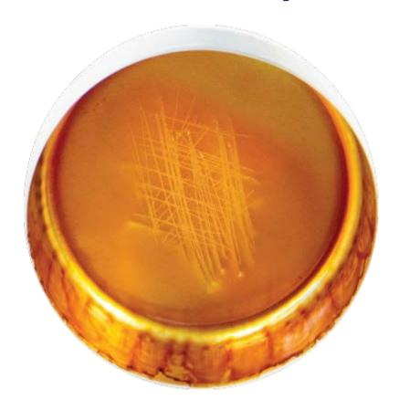
• The samples <u>without</u> NA-LUBE KR-019 created a thin, hard varnish on the metal surface and were not self-healing when scratched.
