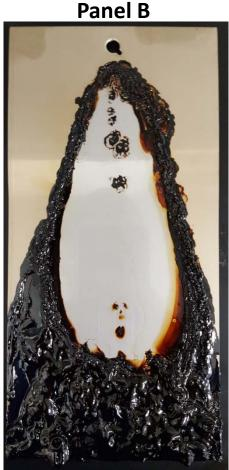
Closed Coke Pattern Failed at 230°C
