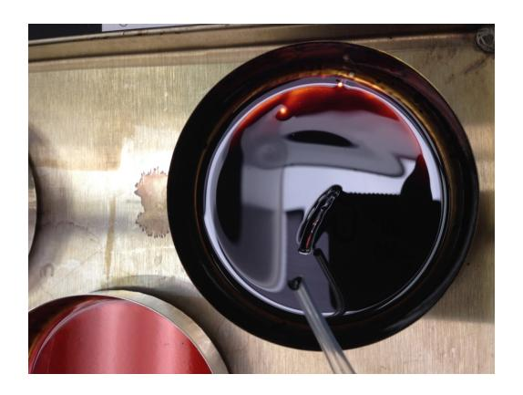
The viscosity of the samples that <u>contain</u> NA-LUBE KR-019 increased after being heated, but the remaining samples were self-healing when scratched.
